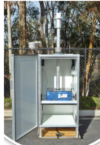
Monitoring shelter and particulate matter sampler
